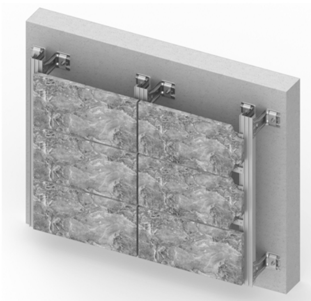
9) Stone facade with glued, invisible buckles
