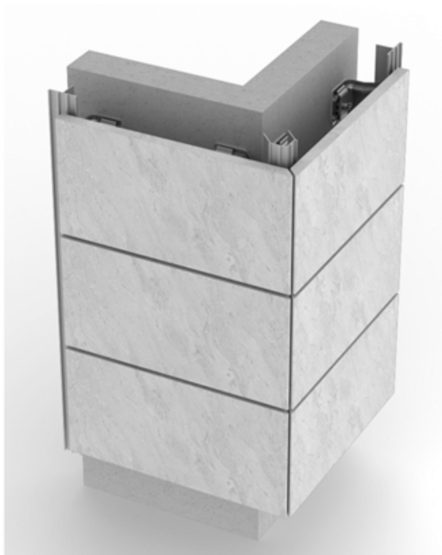
(13) Corner juncture of stone facade
