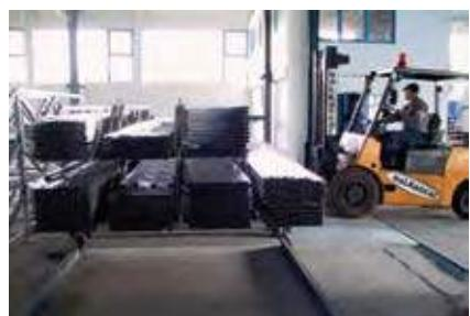
After extrusion, ageing and final quality control, aluminium profiles are stored on a special, custom made shelves that allow separation between different groups and profile types un the warehouse. Further preparation, storage, packaging and transport are different for each of available surface treatments.
