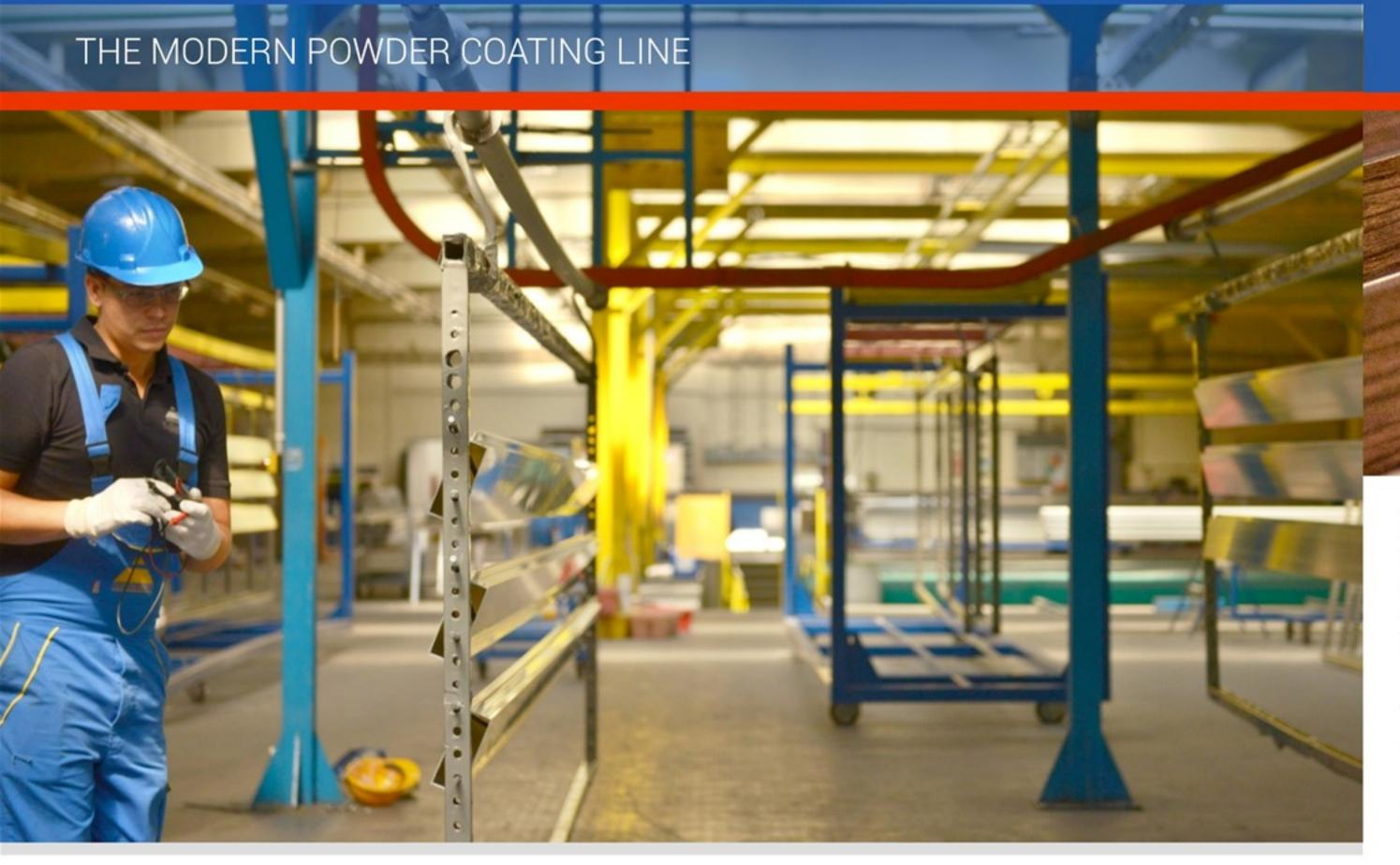
Beside standard powder coating options, the wood effect coating is a particularly interesting option for architects and discerning clients when it comes to aluminum profiles. This is a separate process that requires coating with special sublimation powders and application of special wood colored foils to the aluminum profiles. After that, the profiles are vacuumed and baked in a special oven to achieve a "wood effect" on aluminium profiles to complete this "eco friendly" process.
